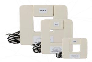
Split-core current transformers are designed to meet the growing demand for installations into existing electrical networks. The Split-core allows installation without disconnecting cables or busbar circuits and hence ideal for retrofitting. They are used for electrical load surveys, energy management systems, sub- metering etc., in conjunction with kilowatt-hour, demand, power factor meters; current transducers or sensing relays.
