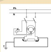
...coil  $K_2$  is excited, the contacts open and the equipment is automatically switched OFF
