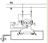
Therefore no current is induced in coil  $K_1$ , and coil  $K_2$  is not excited. The contacts do not open. The equipment operates normally
