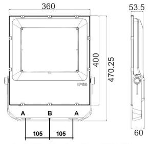
A = SLOTS, 40mm Lg. x 10mm WIDE - 2 Nos. B = DIA 12.5mm HOLE - 1 No.
