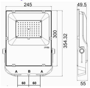
A = SLOTS, 40mm Lg x 10mm WIDE - 2 Nos. B = DIA 12.5mm HOLE - 1 No.
