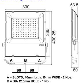
Nominal dimensions in mm Tolerance +/-5 (Except mtg. Hole)
