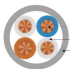
Solid bare Copper Conductor HDPE Insulation
