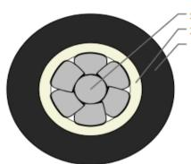
Stranded Aluminum Conductor XLPE Insulation Extruded PVC Type ST2 Outer Sheath
