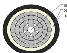
"Stranded Aluminum Conductor "XLPE Insulation "Extruded PVC Type ST2 Outer Sheath
