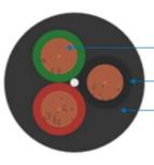
Flexible bunched Copper Conductor
