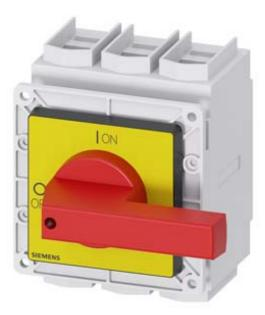
SENTRON, Switch disconnector 3LD, emergency switching-off switch, 3- pole, lu=250 A, operating power / at AC-23 A 400 V: 132 kW, front-mounted, knob-operated mechanism, red/yellow, 4-hole mounting of the handle
