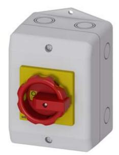
SENTRON, Switch disconnector 3LD, emergency switching-off switch, 3- pole, lu: 16 A, operating power / at AC-23 A 400 V: 7.5 kW, Molded plastic encapsulation for metric cable gland, rotary operating mechanism, red/yellow
