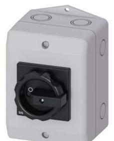
SENTRON, Switch disconnector 3LD, main switch, 3-pole, Iu: 25 A, Operating power / at AC-23 A at 400 V: 9.5 kW, molded-plastic encapsulation for metric cable gland, rotary operating mechanism, black
