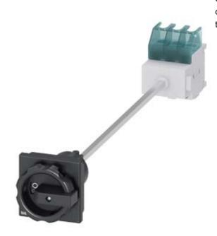
SENTRON, Switch disconnector 3LD, main switch, 3-pole, lu: 32 A, Operating power / at AC-23 A at 400 V: 11.5 kW, floor mounting with door coupling, rotary operating mechanism, black, 4-hole mounting of the handle
