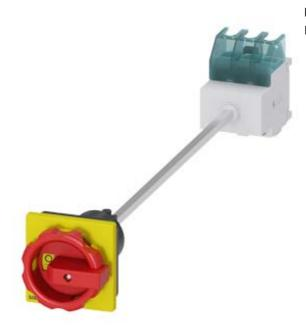
SENTRON, Switch disconnector 3LD, emergency switching-off switch, 3- pole, Iu: 32 A, operating power / at AC-23 A 400 V: 11.5 kW, floor mounting with door coupling, rotary operating mechanism, Red / yellow, 4-hole mounting of the handle
