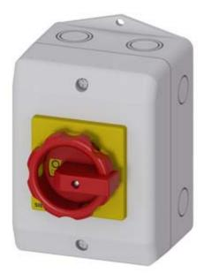
SENTRON, Switch disconnector 3LD, emergency switching-off switch, 3- pole, lu: 32 A, operating power / at AC-23 A 400 V: 11.5 kW, molded-plastic encapsulation for metric screw connection, 1 NC, 1 NO, rotary operating mechanism, red/yellow
