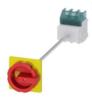
SENTRON, Switch disconnector 3LD, emergency switching-off switch, 3- pole, lu: 63 A, operating power / at AC-23 A 400 V: 22 kW, floor mounting with door coupling, rotary operating mechanism, Red / yellow, 4-hole mounting of the handle
