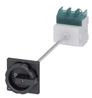
SENTRON, Switch disconnector 3LD, main switch, 3-pole, Iu: 100 A, Operating power / at AC-23 A at 400 V: 37 kW, floor mounting with door coupling, rotary operating mechanism, black, 4-hole mounting of the handle
