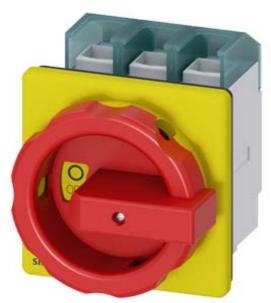
SENTRON, Switch disconnector 3LD, emergency switching-off switch, 3- pole, lu: 125 A, operating power / at AC-23 A 400 V: 45 kW, front-mounted, rotary operating mechanism, Red / yellow, 4-hole mounting of the handle
