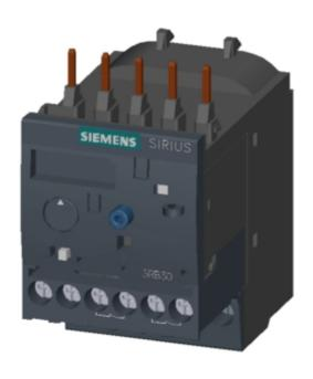
Overload relay 1...4 A for motor protection Size S00, Class 10E Contactor mounting Main circuit: Screw Auxiliary circuit: Screw Manual-Automatic-Reset
