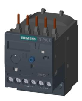
Overload relay 0.1...0.4 A for motor protection Size S00, Class 10E Contactor mounting Main circuit: Screw Auxiliary circuit: Screw Manual-Automatic-Reset
