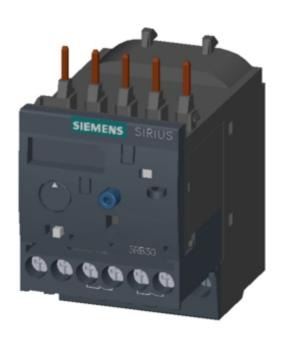
Overload relay 3...12 A for motor protection Size S00, Class 10E Contactor mounting Main circuit: Screw Auxiliary circuit: Screw Manual-Automatic-Reset
