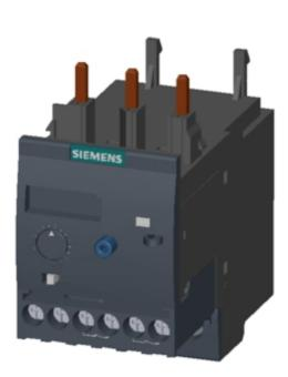
Overload relay 0.32...1.25 A for motor protection Size S0, Class 10E Contactor mounting Main circuit: Screw Auxiliary circuit: Screw Manual-Automatic-Reset
