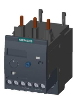
Overload relay 1...4 A for motor protection Size S0, Class 20 Contactor mounting Main circuit: Screw Auxiliary circuit: Screw Manual-Automatic-Reset
