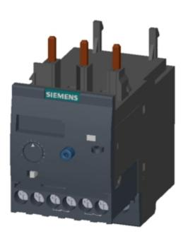
Overload relay 6...25 A for motor protection Size S0, Class 20E Contactor mounting Main circuit: Screw Auxiliary circuit: Screw Manual-Automatic-Reset
