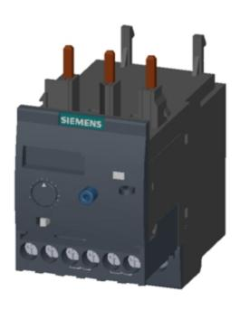
Overload relay 3...12 A for motor protection Size S0, Class 20E Contactor mounting Main circuit: Screw Auxiliary circuit: Screw Manual-Automatic-Reset
