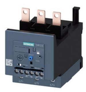
Overload relay 12.5...50 A Electronic For motor protection Size S3, Class 10E Contactor mounting Main circuit: Screw Auxiliary circuit: Screw Manual-Automatic-Reset
