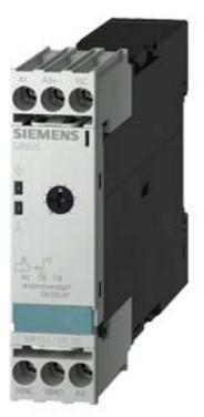
Timing relay, electronic Phase-out product! For further information, contact our sales department ON delay 1 CO contact, 1 time range 0.5 s...10 s 24, 200...240 V AC and 24 V DC at 50/60 Hz AC with LED, screw terminal
