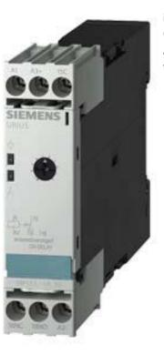
Timing relay, electronic Phase-out product! For further information, contact our sales department ON delay 1 CO contact , 1 time range 0.5 s...10 s 24, 100...127 V AC and 24 V DC at 50/60 Hz AC with LED, screw terminal
