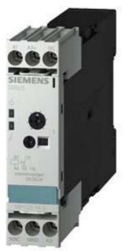
Timing relay, electronic Phase-out product! For further information, contact our sales department ON delay 1 CO contact 15 time ranges 0.05 s...100 h 24, 100...127 V AC and 24 V DC at 50/60 Hz AC with LED, screw terminal
