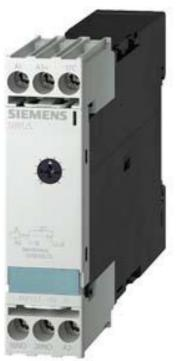
Timing relay, electronic Phase-out product! For further information, contact our sales department w. star-delta (wye-delta) function 1 NO contact, delayed 1 NO contact, instantaneous 1 time range 3...60 s 24 V AC/DC and 200...240 V AC at 50/60 Hz AC Screw terminal
