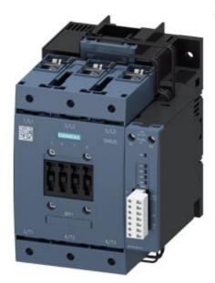
Power contactor, AC-3 115 A, 55 kW / 400 V AC (50-60 Hz) / DC operation 200-277 V UC Auxiliary contacts 1 NO + 1 NC 3-pole, Size S6 with box terminals Drive: electronic with PLC / SIMOCODE interface and RLT signal
