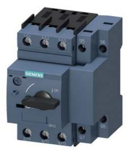
CIRCUIT-BREAKER SZ S00, FOR MOTOR PROTECTION, CLASS 10, W. OVERLOAD RELAY FUNCTION A-RELEASE1.8...2.5A, N-RELEASE33A, SCREW CONNECTION, STANDARD SW. CAPACITY
