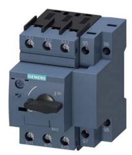
CIRCUIT-BREAKER SZ S00, FOR MOTOR PROTECTION, CLASS 10, W. OVERLOAD RELAY FUNCTION A-RELEASE 2.2...3.2A, N-RELEASE42A, SCREW CONNECTION, STANDARD SW. CAPACITY
