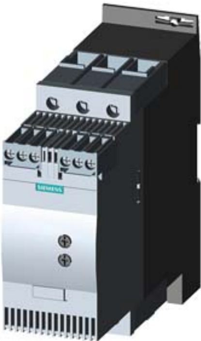
SIRIUS SOFT STARTER, SIZE S2, 45A, 22KW/400V, 40 DEGREES, 200-480V AC, 24V AC/DC, SCREW TERMINALS
