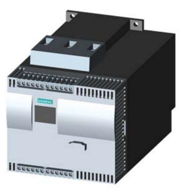
SIRIUS SOFT STARTER, VALUES WITH 500 V, 40 DEG., STANDARD: 77A, 45KW, INSIDE-DELTA CIRCUIT 3: 133A, 90KW, 400-600 V AC, 230 V AC, SCREW TERMINALS
