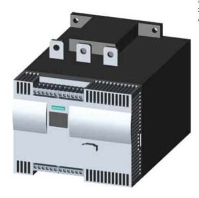
SIRIUS soft starter Values at 460 V, 50 °C Standard: 280 A, 200 hp Inside-delta: 485 A, 400 hp 200-460 V AC, 115 V AC Screw terminals
