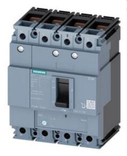
circuit breaker 3VM1 IEC frame 160 breaking capacity class S Icu=36kA @ 415V 4-pole, line protection TM220, ATFM, In=100A overload protection Ir=70A...100A short-circuit protection Ii=10 x In N conductor protection 100% nut keeper kit
