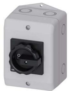
SENTRON, Switch disconnector 3LD, main switch, 3-pole, lu: 16 A, Operating power / at AC-23 A at 400 V: 7.5 kW, molded-plastic encapsulation for metric screw connection, 1 NC, 1 NO, rotary operating mechanism, black
