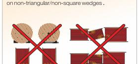
Allow the drums to roll at any cost. Stack the drums
